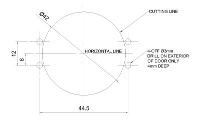
Installation Template of door viewer. Please check the dimensions of the template before you cut to size.
