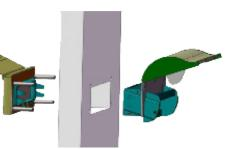
**STEP 5** Secure the back plate to the door using 4 x 29mm bolts.
