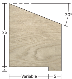
Glazing bead For timber screens.
