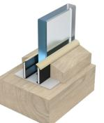
The expansion allowance should be as per the glass manufacturers certificates. As a general rule there should be a minimum gap of 4mm to each glass edge. Hardwood or noncombustible setting blocks may be used along the bottom edge only in order to facilitate this.
