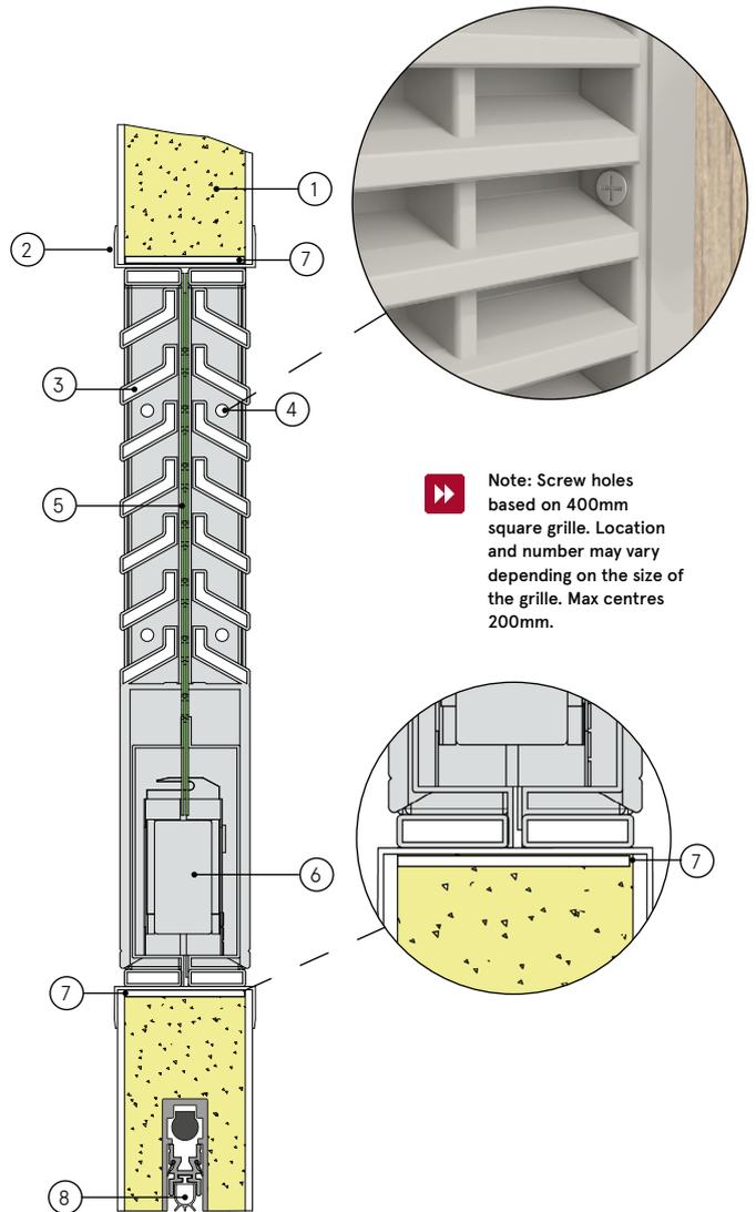
**Note:** Screw holes based on 400mm square grille. Location and number may vary depending on the size of the grille. Max centres 200mm.
