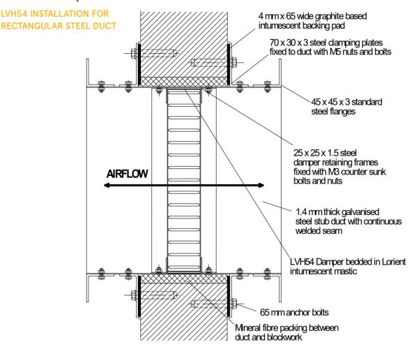
LVH54 installation for rectangular steel duct.
