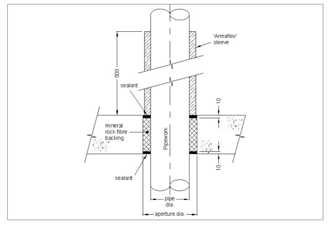
A.3.1 Penetration seal with metal pipe including combustible insulation
