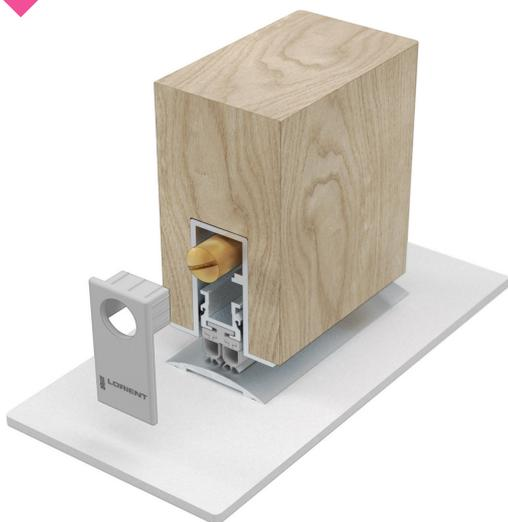
LAS8012 si & LAS8013 si are heavy-duty aluminium drop seals featuring twin gaskets for excellent acoustic performance. Both seals feature a high efficiency mechanism, which lift the seals clear of the floor as soon as the door is opened by a few millimetres. They require no power connection.
