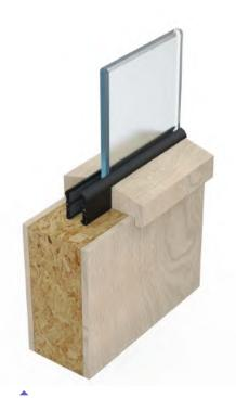
Example of a 30 minute glazing system for a glazed aperture
