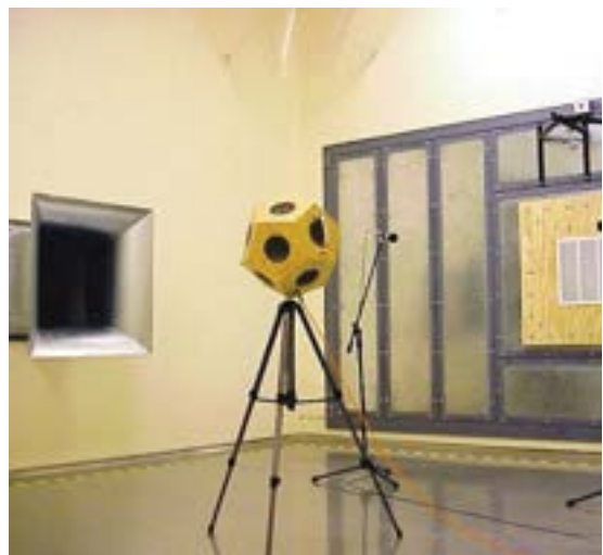
Images: NCRL Acoustic and pressure loss test
