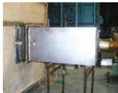
AS1530.4 2014 air transfer grille testing
