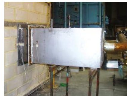
AS1530.4 2014 air transfer grille testing
