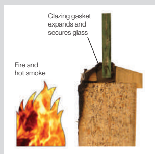
System-36 PLUS and System-63Ø operating in 'hot' condition
