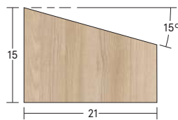
Glazing bead For unrebrated screen frames.
