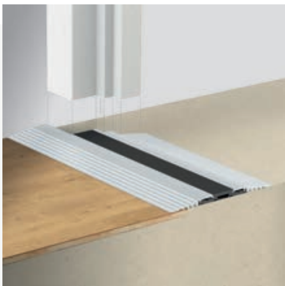
Planet F140 click-threshold with reduced height, ideal for renovations since no floor strike required (image: installation between frame)
