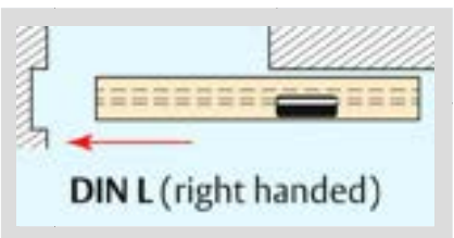
Sliding door closing to the left = DIN L
