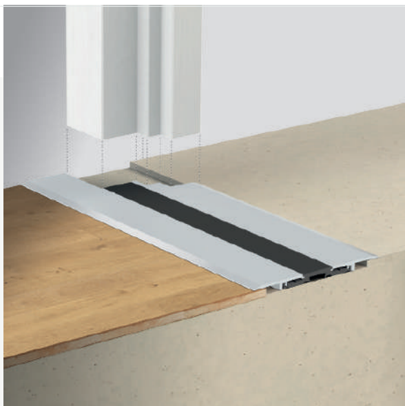
Planet F120 click-threshold for extremely flat transition between inside and outside (image: installation between frame)
