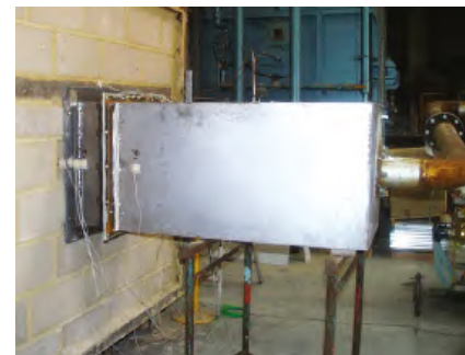
AS1530.4 2014 air transfer grille testing
