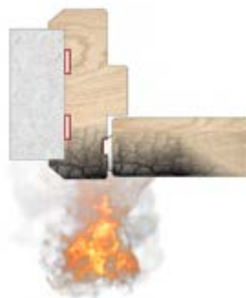
Combined seals provide an effective barrier to the passage of fire and hot smoke
