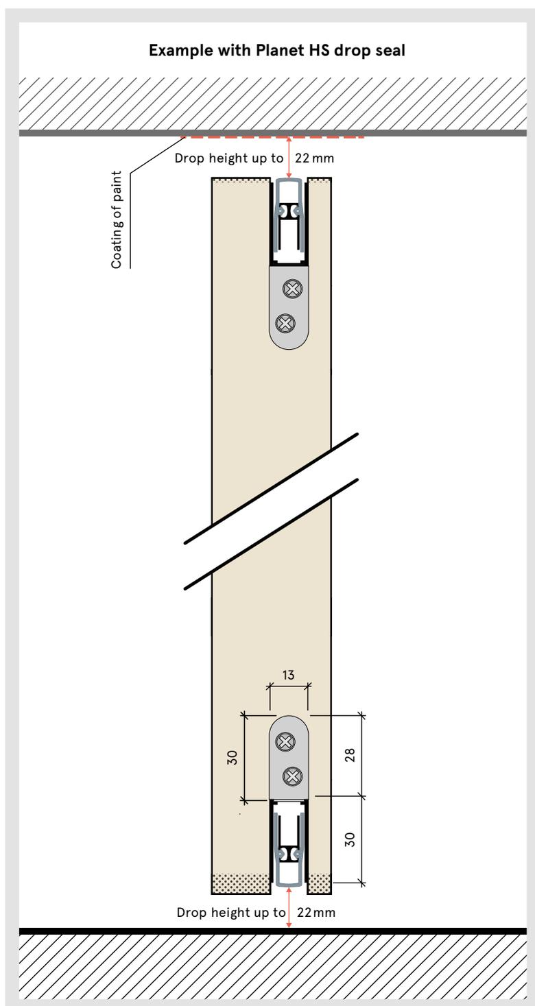
The Planet silicone lip leaves no traces, but the last coating of paint on the ceiling in the zone of the seal must be smooth and non-abrasive.
