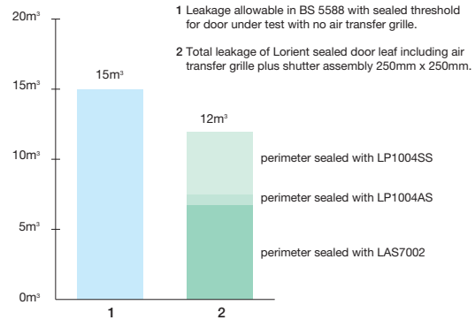
Total smoke leakage of door leaf and damper / air transfer grille related to door perimeter
