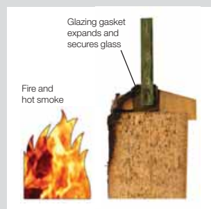
System-36 and System-63Ø operating in 'hot' condition
